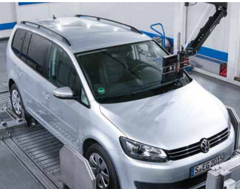
The MAHLE test vehicle with monovalent natural gas downsizing engine on the chassis dynamometer
