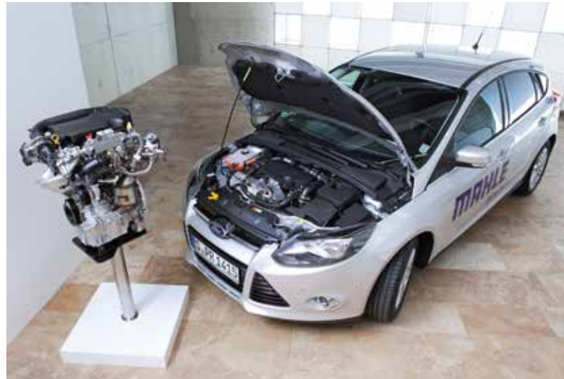
The MAHLE EGR test vehicle with large-scale production gasoline engine and applied high- and low-pressure EGR system
