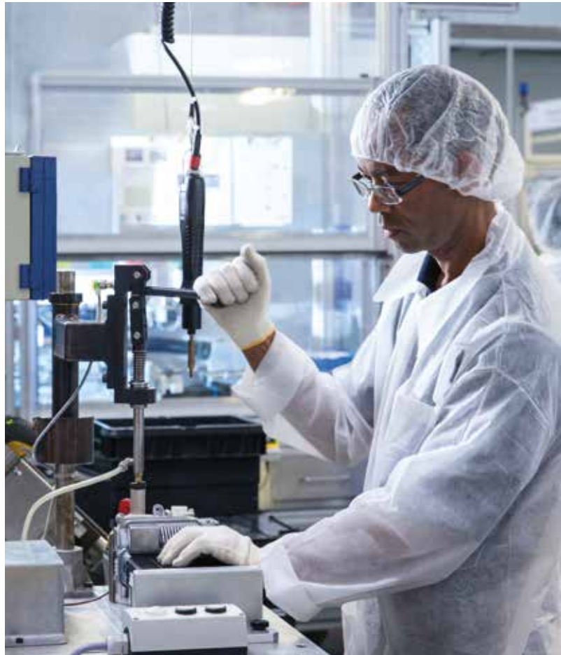
Mounting a regulator on a PTC heater with integrated leak testing
